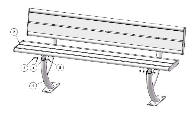
Recommended Surface Mount Hardware: 3/8" x 3-1/2" Concrete Expansion Anchor Bolts (Not Included)
