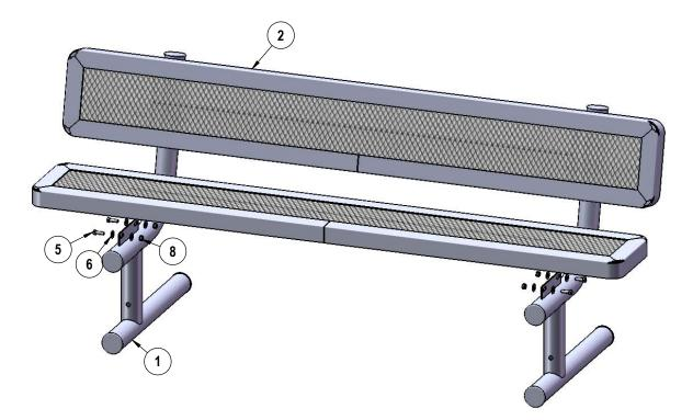
Attach the seat planks as shown using specified hardware.
