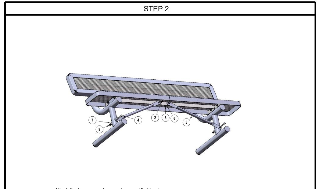
Attach the braces as shown using specified hardware.
